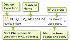
The lower left field displays the characteristic by which the Discovery list is currently sorted. In the image above, the list is sorted by MAC address. See Discovery Sorts in this topic for more about sorting.
