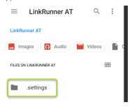
If desired, you can manually edit this file on the LRAT unit, or you can create a new authname.txt file on a PC and import it onto your unit in the same file location. (You can also push authname.txt files from Link-Live to your test unit.)
