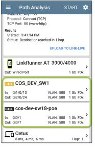
The LRAT is able to identify these Layer 2 switches and their interfaces because it has configured SNMP access to the switches.
