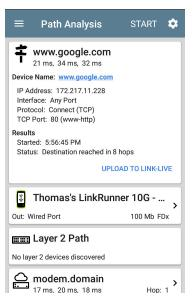
Like AutoTest, Path Analysis results are presented on cards. The top card shows the main test details, the second card shows information for the source device (your
