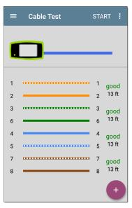
When a cable has no detected faults, "good" is shown next to each pair above the length measurement. Cable tests that detect a "split" or "open" in the cable also display the corresponding words.
