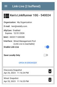
The buffered files displayed automatically upload to Link-Live.com once your LRAT connects to an active network.
