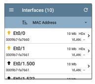
Tap an Interface row to open a new Discovery Details screen for that Interface.
