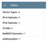
The Filters screen displays the number of devices or domains discovered for each category. Tap a category name to select filters by checking the boxes. The main Discovery screen shows only those devices or IDs that fall under your chosen filter parameters.
