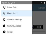
Tap Flash Port to open the Flash Port screen. If the connection to the switch is good, a blue line connects a test unit icon to a switch icon.
