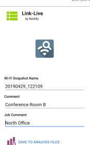
The Link-Live sharing screen for a screenshot or other image allows you to attach it to the most recently run test result on the Results page, or to the Uploaded Files page on Link-Live.com.
