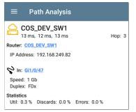
Tapping the <u>blue linked</u> switch name opens a <u>Discovery Details screen</u> for the switch, where the user can investigate the cause of the Warning.
