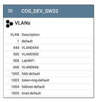
The VLANs Details screen also shows the description with each VLAN ID.
