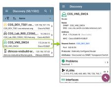
The available data and actions on the Details screens vary significantly depending on the device type, connections, and data the LRAT was able to discover. In other words, only the discoverable information for each device is shown on the Details screen.
