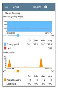
UDP Packet Loss Up and Down graphs: When running a UDP protocol test, the iPerf results also display graphs and tables of Packet Loss. Values for the number and percentage of packets lost are displayed in the table below the
