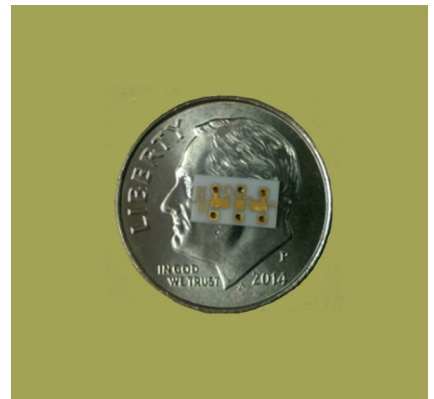
▲ Fig. 7 Microminiature 5.83 GHz C-Band filter.
