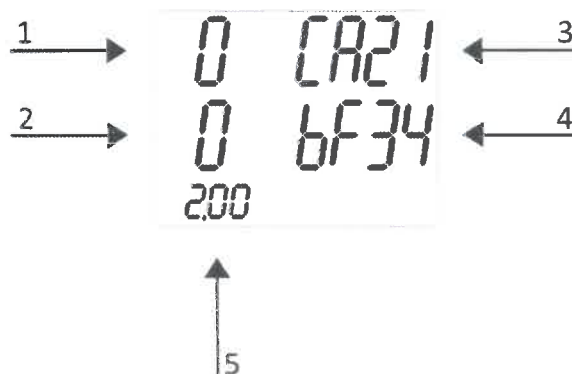
Figure 2: WM3M4C/WM3M4 identification of MID relevant counters and FW identification
