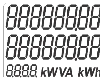
Figure 6: LCD segment test
