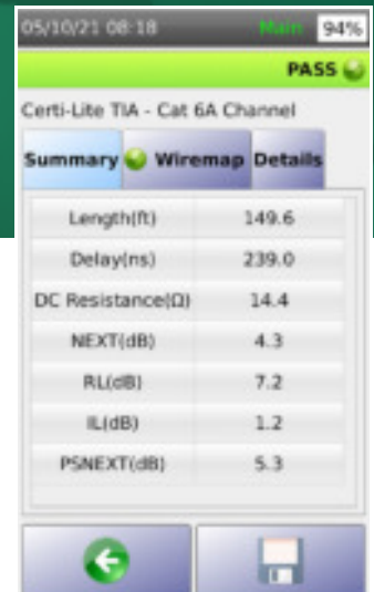
Figure 4 - Certi-Lite Autotest result can be obtained with Remote IDs. Click on Details tab to drill into each test result. Test Results can be stored in tester memory for later upload to the included PC based TestDataPro, or immediately with the included TestDataPro Cloud via wired or wireless network connection.
