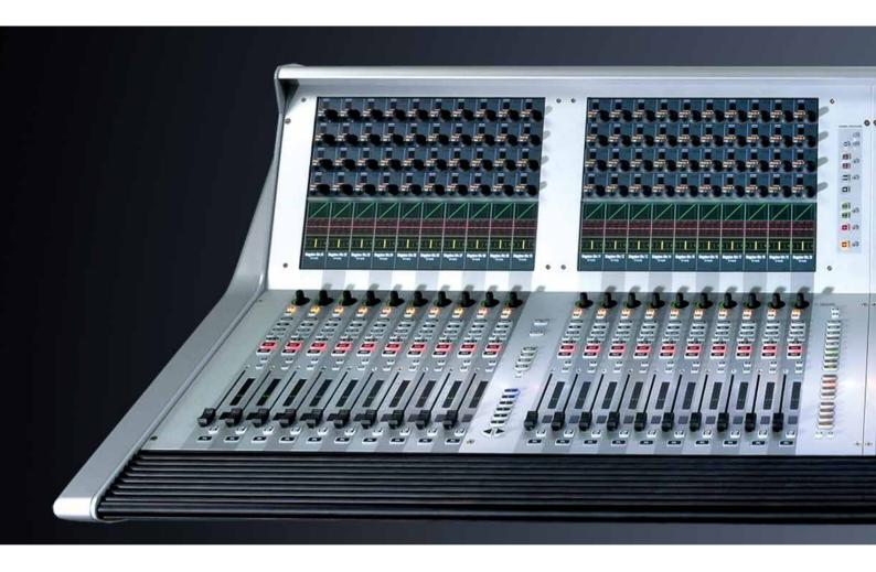
Control requirements for outputs differ from those for inputs in several important ways. Excellent metering and fast adjustment of the output channel levels themselves is essential. But it is often the input channels that contribute to the master that are important to the user. Usually the level control of the contributing channels is handled via the input channel strips, but the Studer Vista 5 SR offers a unique and revolutionary operational concept for controlling outputs. The Control
