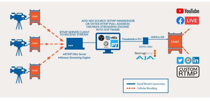
RTMP MiniServer provides RTMP URLs that are entered into LiveU Solo's web portal to send feeds to it. Then, it converts the received feeds into NDI (Network Device Interface) sources that automatically appear in any software that supports NDI. This protocol enables simple sharing of video sources across a network.
