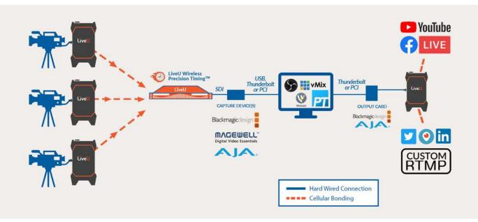
In the diagram, 3 remote LU300 transmission units (which offer 4 cell modems + Wi-Fi + Ethernet) are feeding video back to an LU2000 quad output server located anywhere in the world. Output to the server is a simple process of looking at the encoder's screen and selecting a preconfigured output channel that corresponds with a specific SDI output port on the server.
