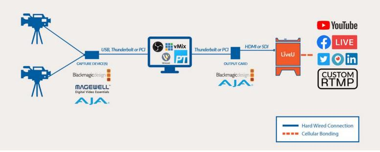
In the diagram, see the workflow components to the right of the computer. Most switcher softwares offer compatibility with dedicated output cards for true high-resolution video out via SDI or HDMI. Blackmagic and AJA external or internal output cards which connect to computer with Thunderbolt or PCI are recommended. Output via direct HDMI connection from computer into LiveU Solo is not advised, as this type of monitor output may not be reliable nor offer full resolution.
