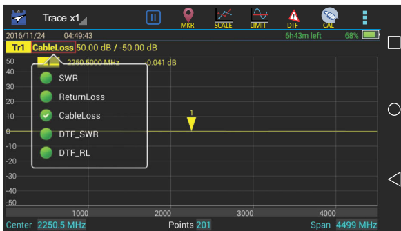
Figure 29 Selecting Cable Loss Measurement
