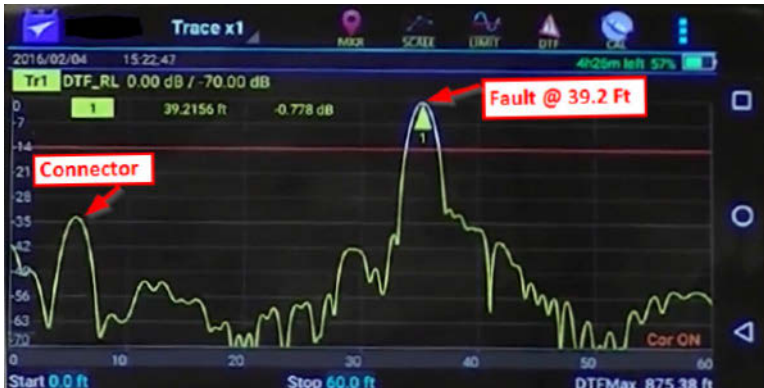
Figure 1 Typical Fault Location Measurement
