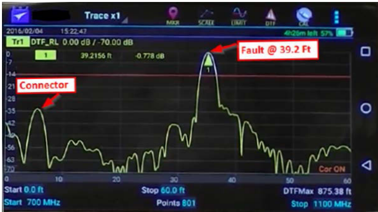
Figure 1 Typical Fault Location Measurement
