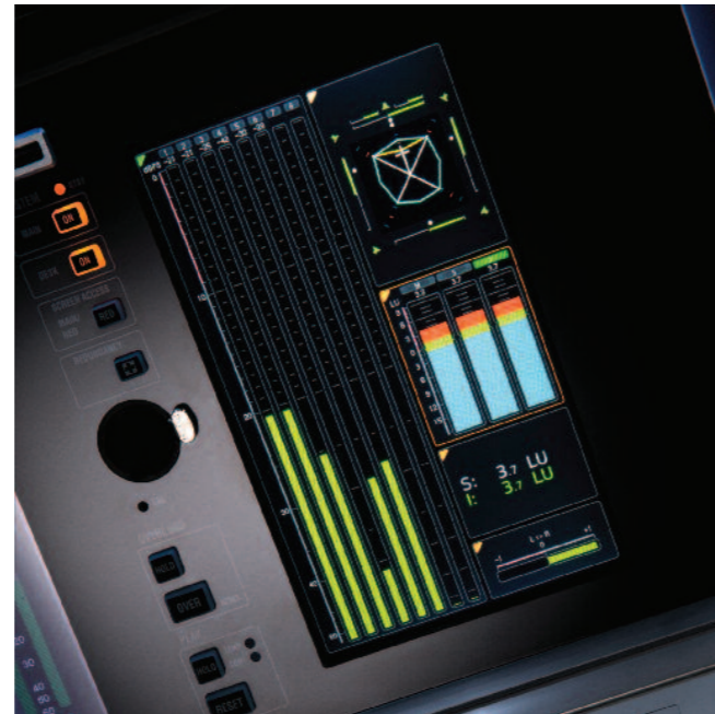
Loudness metering is built right into the console.
