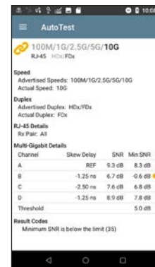
Cabling SNR measurement validates Multi-Gig links
