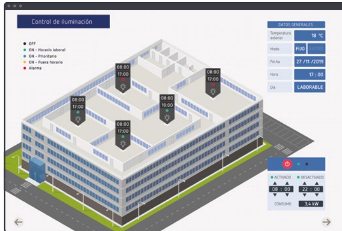
Example of lighting control
