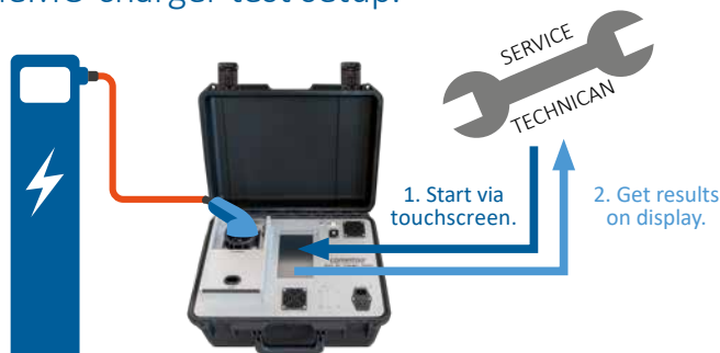
CHAdeMO charger test setup:
