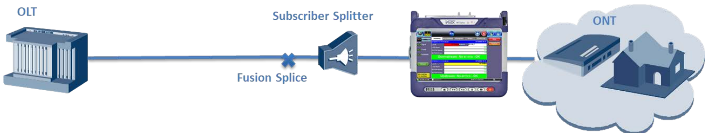
Figure 27: The MTTplus-420 should be connected between the splitter and ONT.
