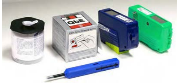
Figure 6: Optical fiber cleaning materials clockwise from left--isopropyl alcohol, lint free soft tissues, connector reel cleaners, and a ferrule cleaner
