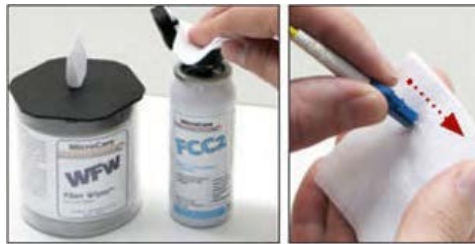
Figure 7: Clean the connector end-face by rubbing it onto a lint-free wipe dampened with isopropyl alcohol
