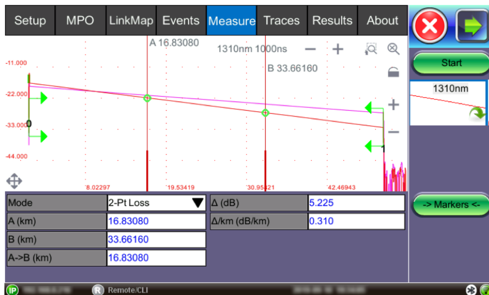
Splice Loss using 2-Point LSA method (MPO)
