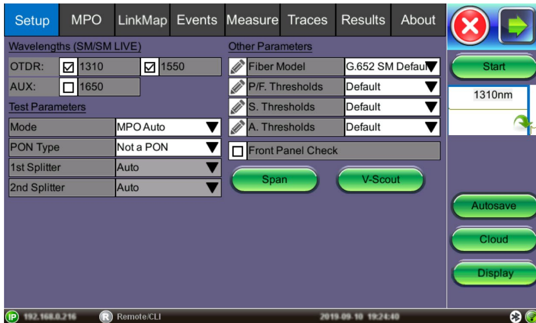
OTDR Screen (with MPO switch connected)
