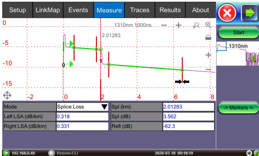
Splice Loss using 5-Point LSA method
