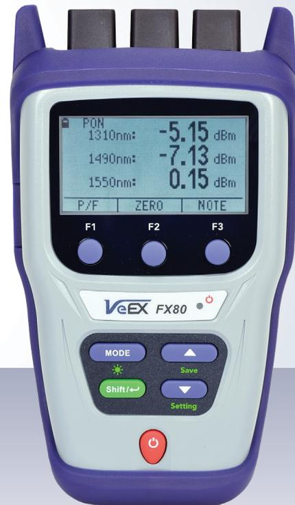
In-line optical power meter for GPON or EPON service activation and troubleshooting. Simultaneously measures downstream signals to the ONT and upstream signal to the OLT.
